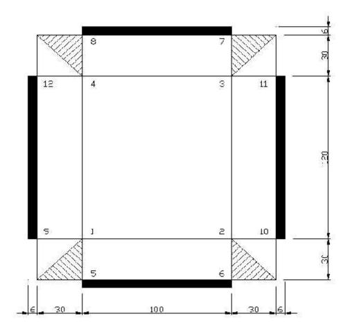
Black portion is to be bend (hem). Hatched portion is to be cut out. All Dimensions are in mm **AIM:** - To make a Square box using G.I Sheet as per the dimension
